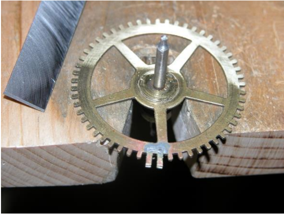
Finished result of inside teeth. Notice equaling file with sanded off safe side and square edge.
