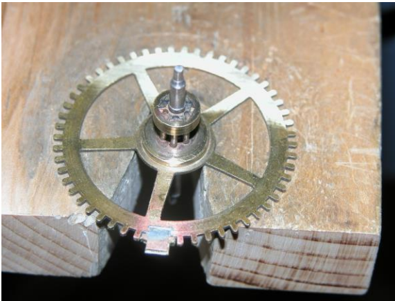
Crosswise file ledge on both outside tooth spaces
